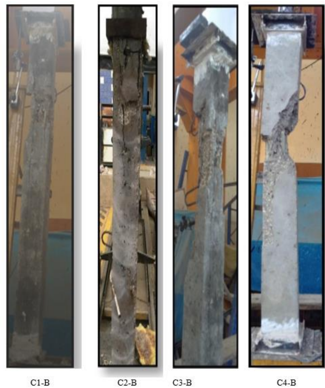
Fig 12 Crack patterns(Group B)
