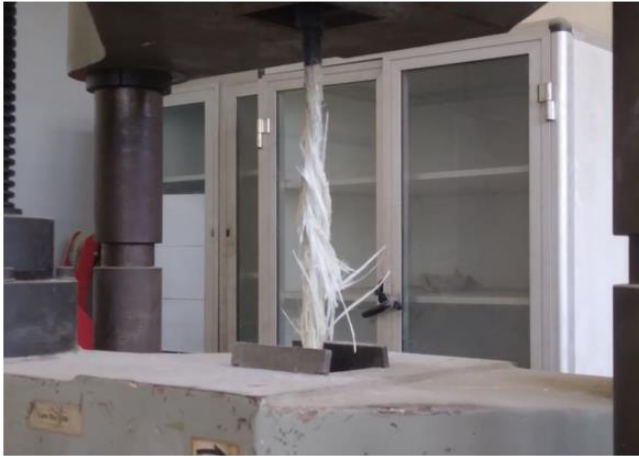
Fig 6 Failure Mode of GFRP bars.
