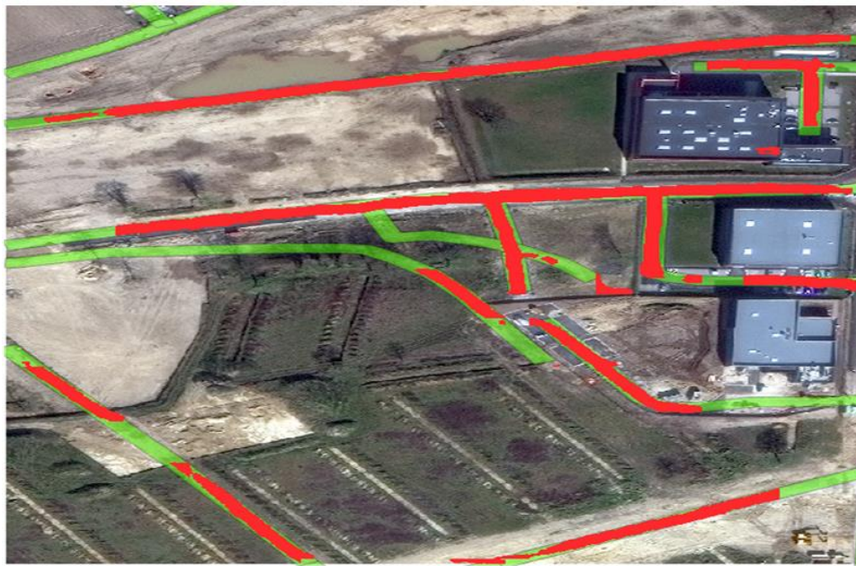
FIGURE 7. Comparison of Ground Truth and Predicted Segments using Multi-Task Road Extractor Model.
