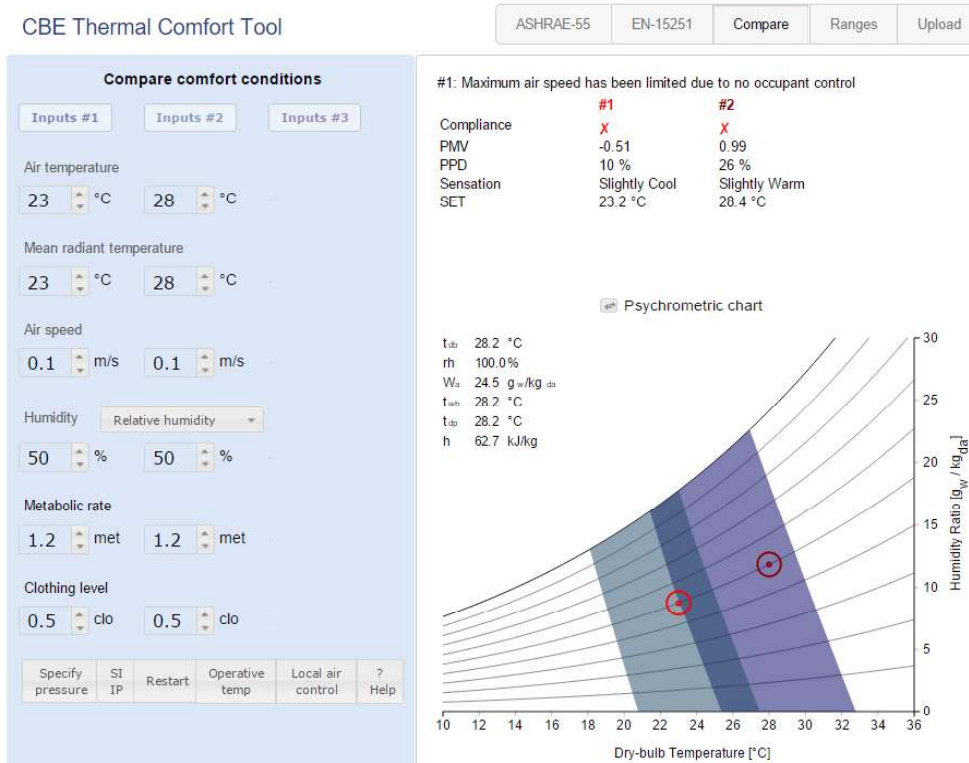
Figure 9: An Example with the application of CBE thermal comfort tool showing the comparison between two different temperatures http://cbe.berkeley.edu: http://cbe.berkeley.edu/comforttool/
