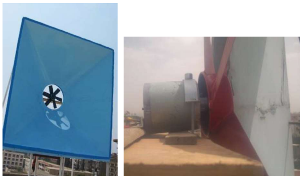
Fig. 1: Final assembly of the wind cube and the generator on its base.
