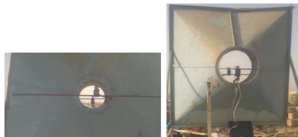
Fig. 2: Fixing the Kestrel 4500 at the inlet of wind cube and Kestrel 4200 at the outlet of wind cube to measure the nozzle efficiency.
