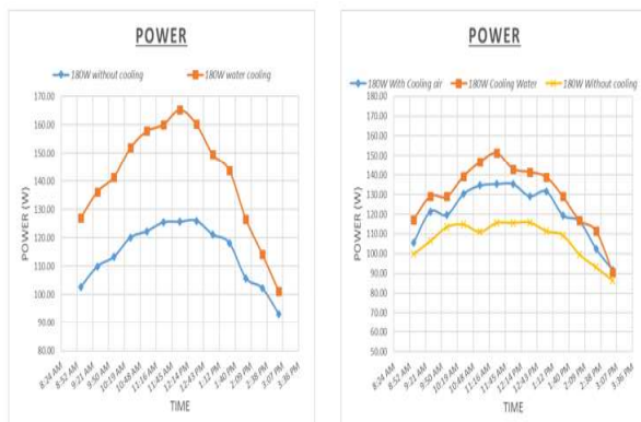
Fig. 29 Effect of cooling in output power of PV
