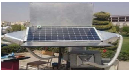
Fig 15 Reflector with DC linear motor
