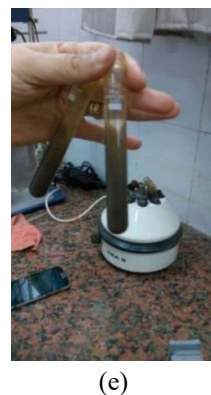
Fig. 4: Chemical treatment of the rice straw: a) diluted HCl 10%, b) adding HCl to the filtered solution, c) centrifuge equipment, d) the formed silica gel, and e) the collected silica gel
