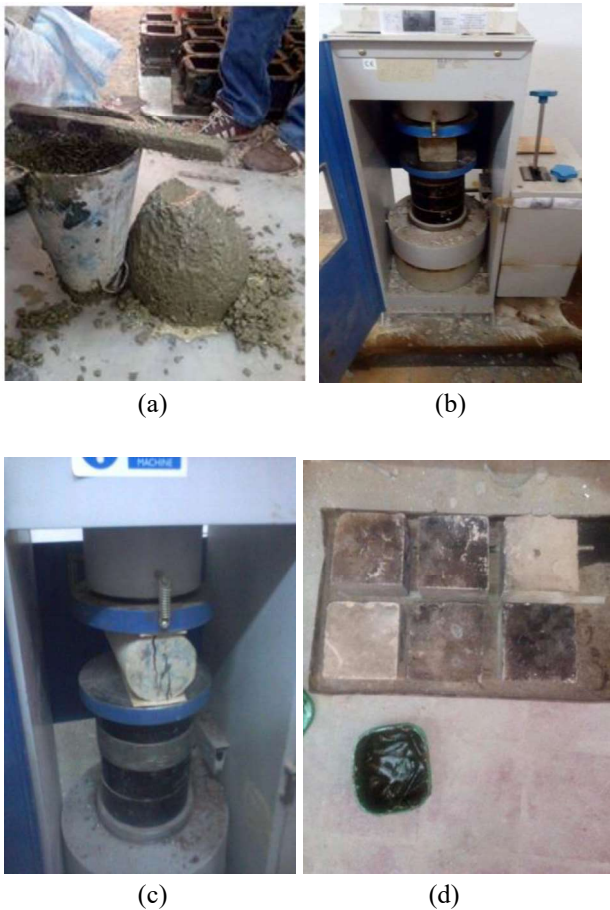
Fig. 6: Performed tests on concrete: a) slump test, b) compression test, c) splitting tensile test, and d) sorptivity test
