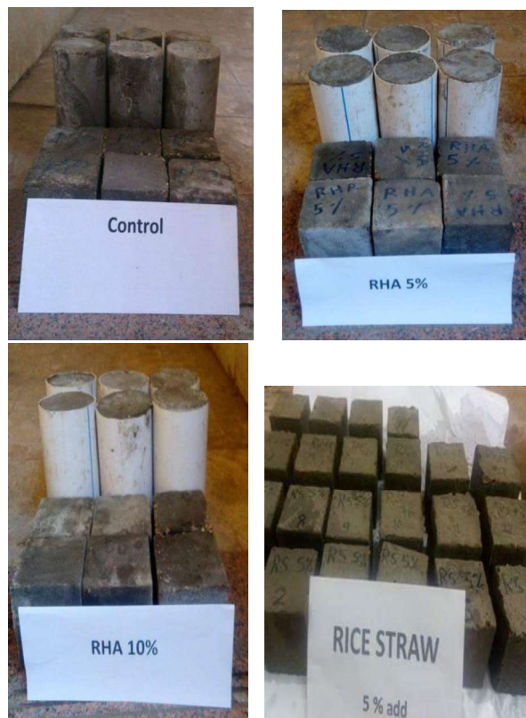
Fig. 5: Specimens prepared from concrete mixes for hardened concrete tests.
