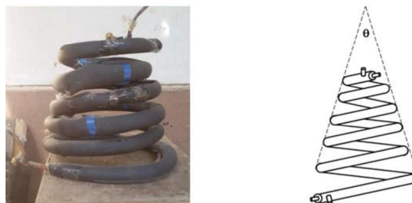
Fig. 3: A photograph and schematic representation of the CCTIT evaporator/condenser.
