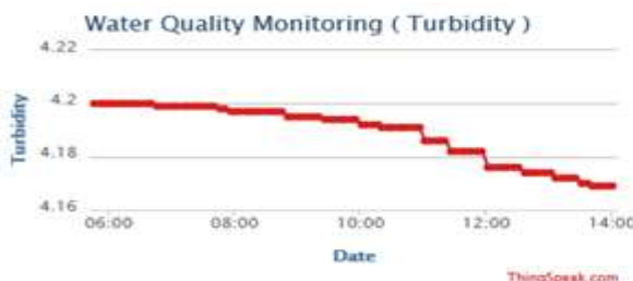
FIGURE 7: Turbidity Sensor Experimental Results with fish inside basin.
