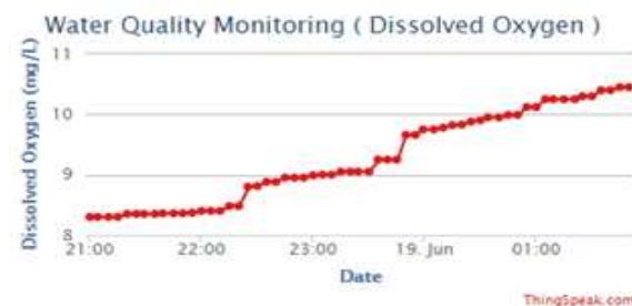
FIG 10: Dissolved Oxygen Sensor Experimental Results without fish inside basin.
