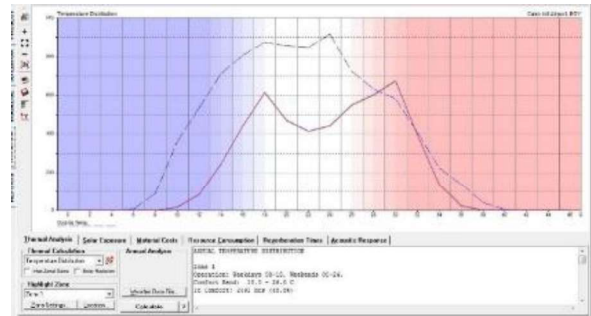
Figure 20: The difference between the temperature inside Room and outside the stadium after add modification Reference: Researcher by using Ecotect Program
