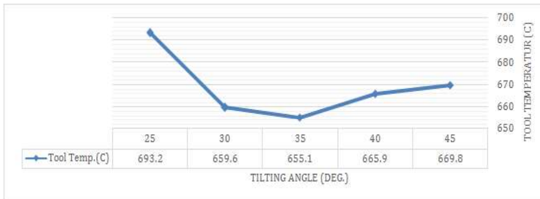
Fig.8 Influence of different tilting angles on thermal behavior using SPRT ( V_c = 85 m/min, f = 0.56 mm/rev, a = 0.53 mm)
