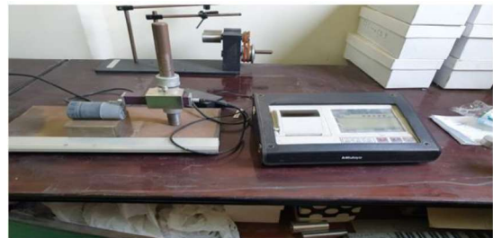
Fig 4. Surface roughness measurement device (MitutoyoSurftest SJ-310)
