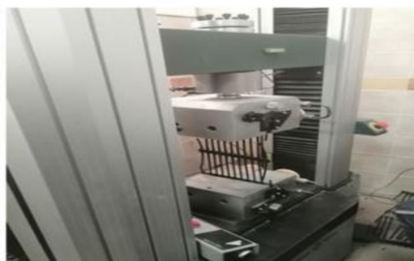
(b) Test of geogrid.
