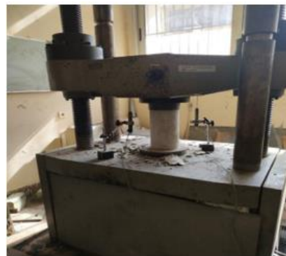
FIG 5. Configuration for testing concrete cylindrical compressive strength
