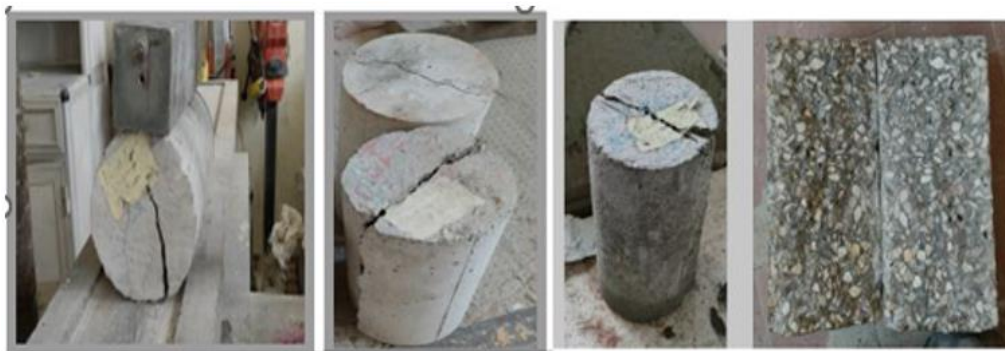
FIG 12. Splitting failure modes for the concrete specimens
