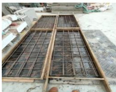
FIG 8. Detailed depiction of the tested slab specimens
