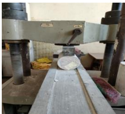
FIG 6. Setup for testing splitting tensile strength of cylinders
