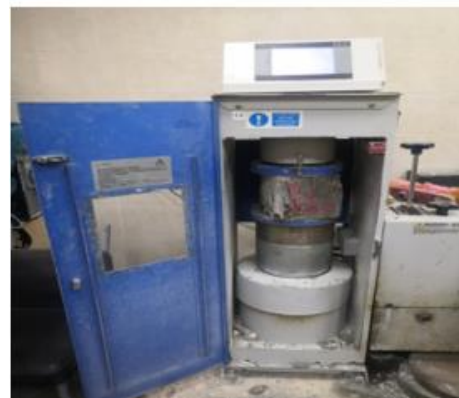
FIG 4. Configuration for concrete compressive strength testing
