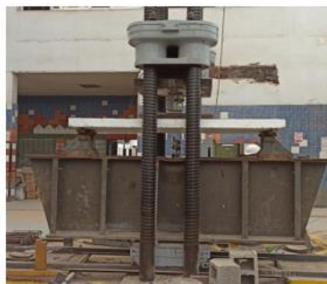
FIG 3. Setup for slab testing
