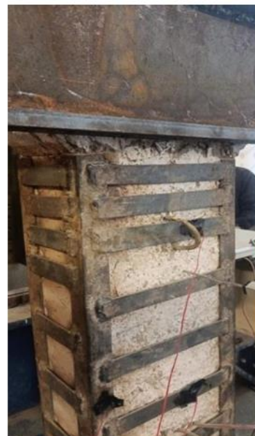
(a) Compression damage of FE model. (b) Crack pattern of tested specimen. Figure 30: Comparison between the crack pattern of the experimental model and its corresponding FE model of C2.
