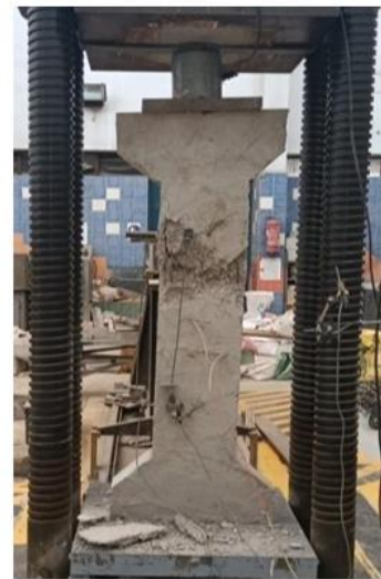
(a) Compression damage of FE model. (b) Crack pattern of tested specimen. Figure 29 Comparison between the crack pattern of the experimental model and its corresponding FE model of C1.
