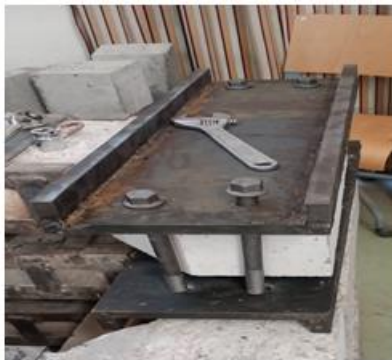
Figure 6: Columns steel head.
