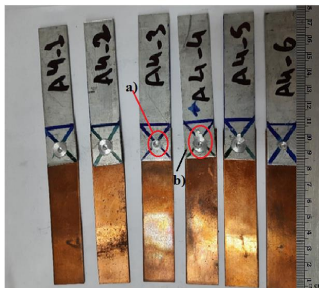
FIG 5. Visual inspection of weld specimens at 1800 rotational speed , 10 seconds dwell time and 0.1mm plunge depth with a) lack of penetration b) excess flashes.
