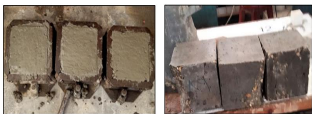
Fig.2 Preparation of Concrete Standard Cubes
