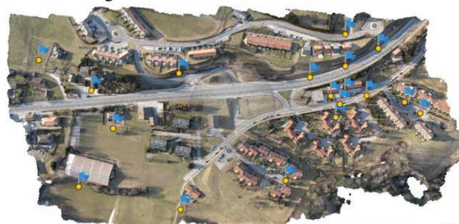
FIG2. The distribution of the ground reference points
