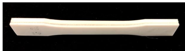
Fig 5. Specimen printed at 210°C failed before yielding where layers were separated
