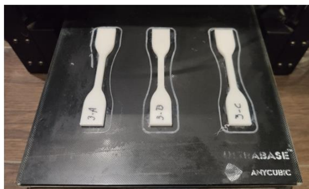
FIG3. Three dog bone specimens are printed consecutively with the same layer height which is indicated by the number. Each number is assigned to a certain layer height while the letter determines whether it is printed on the left region (A), middle region (B) or the right region (C).
