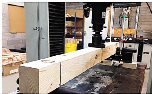
Fig. 5 Model I wooden beam (dimensions in mm) [20]
