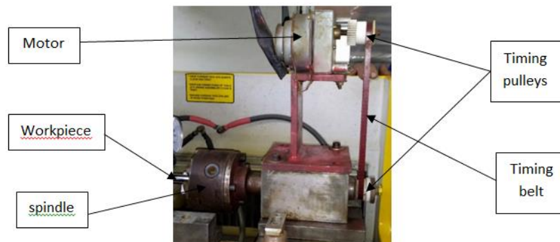
FIGURE 3. Rotating mechanism unit.
