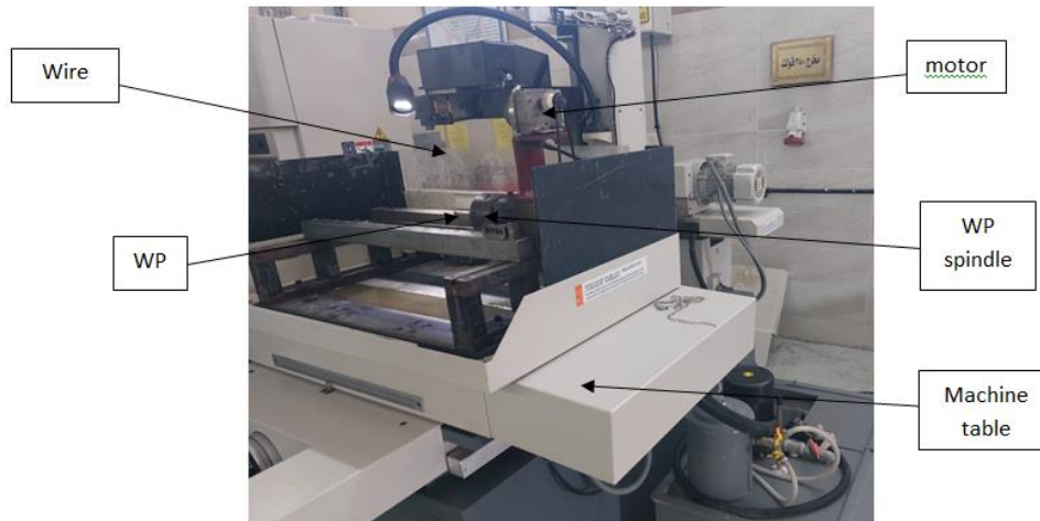
FIGURE 1. SUZHOU BAOMA CNC wire cut EDM DK7740 machine.
