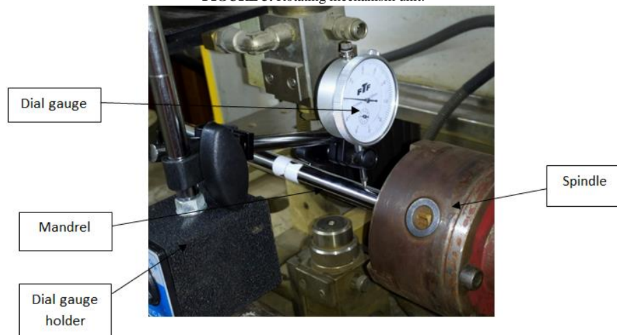
FIGURE 4. Measuring of runout of the spindle.
