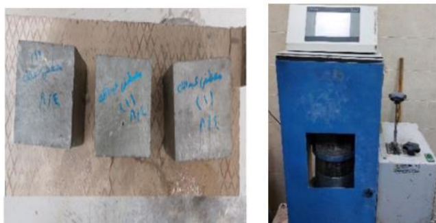
Fig. 2. Concrete cube compressive strength test.
