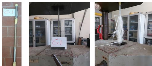
Fig. 3. Tensile testing of GFRP bars.
