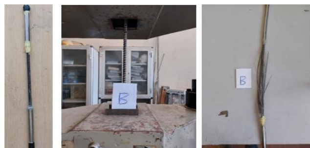
Fig. 3. Tensile testing of GFRP bars.
