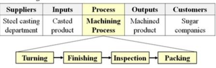
Fig 2. Process description and SIPOC diagram.
