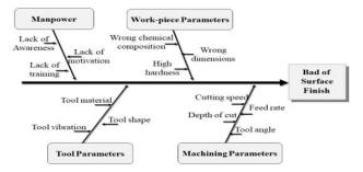
Fig 6. C&E diagram for bad of surface finish
