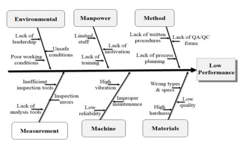
Fig 12. C&E diagram for low process performance.
