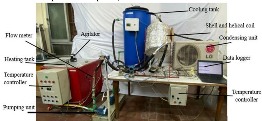
FIGURE 1: Experimental apparatus photo with instrumentations.
