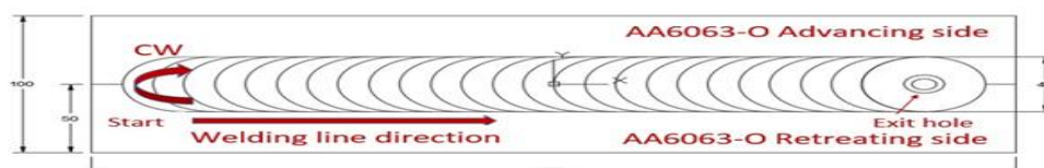
Fig.2. Dimensions of FSW specimen and joint, all dimensions in (mm).
