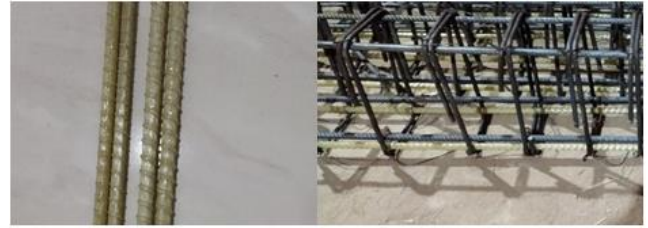
Fig 1. Produced GFRP and Steel Bars
