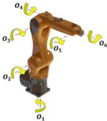
FIGURE 1. Arbitrary Posture for KUKA RR6 R900
