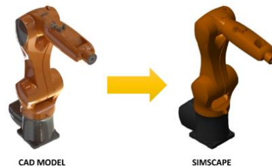
FIGURE 3. KUKA KR6 R900 CAD Model to MATLAB-SIMSCAPE Platform
