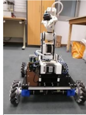
Fig. 2. Fully assembled mecanum wheeled robot.
