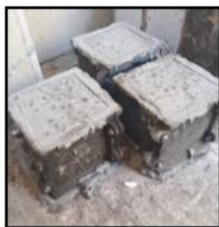
FIGURE 1. Concrete cubes for examined columns.
