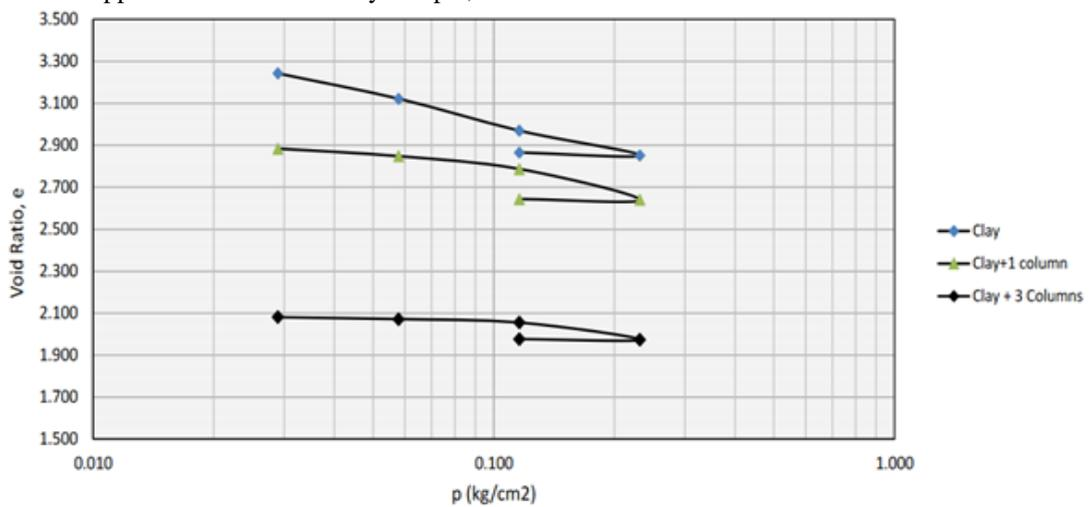
Fig 11: Consolidation Test Results for All Tests
