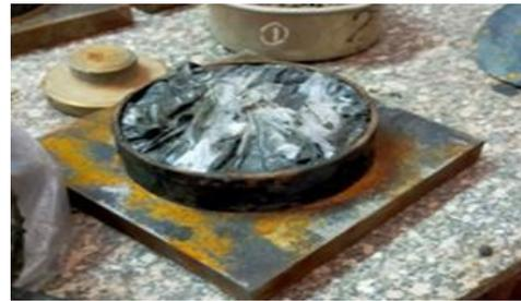
Fig 5: Sample after Wrapping with Thin Plastic Bag
