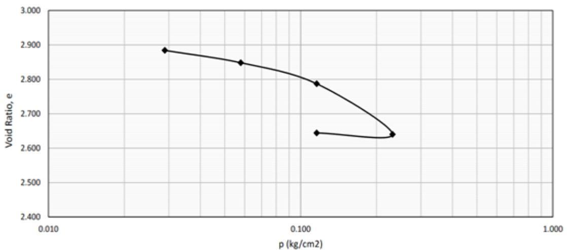
Fig 9: Consolidation Test Results for Clay Treated with One SC Column
