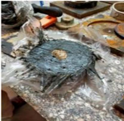
Fig 3: Soft Clay Treated with One SC column
