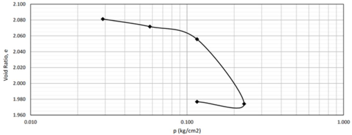
Fig 10: Consolidation Test Results for Clay Treated with Three SC Column
