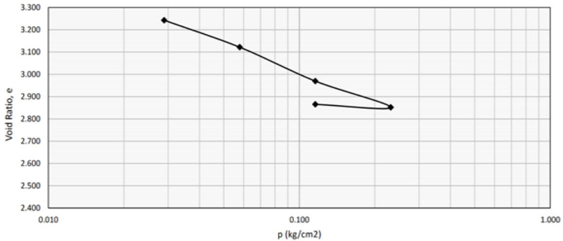
Fig 8: Consolidation test Results for Clay With no Treatment
