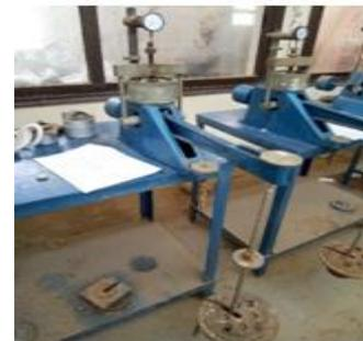
Fig 7: Loading Frame and Dial Gauge
