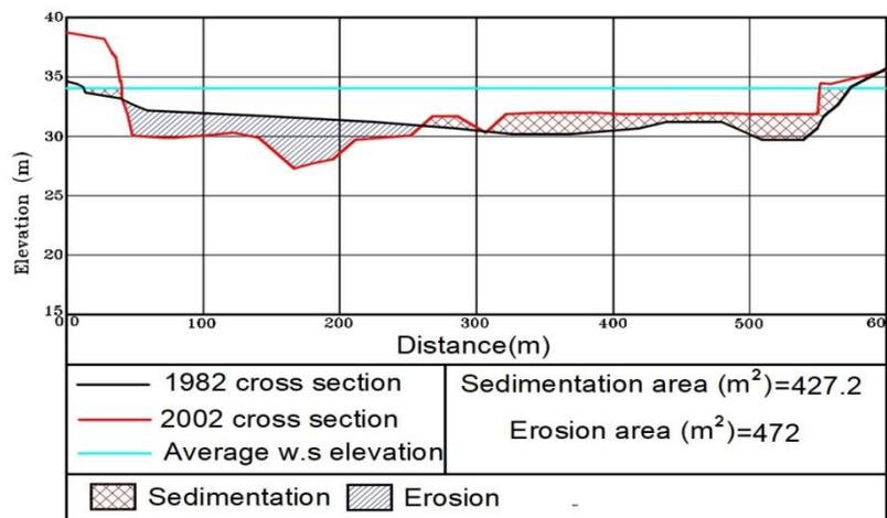
**Fig 4.**The deposition and scour at a cross-section at km 684.450 from AD.
