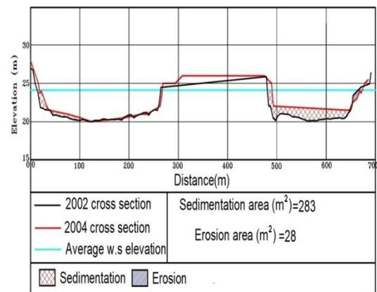
**Fig 12.** The deposition and scour at a cross-section at km 810.280 from AD.
