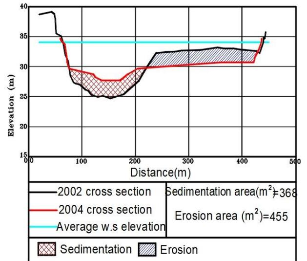
**Fig 5.** The deposition and scour at a cross-section at km 684.690 from AD.
