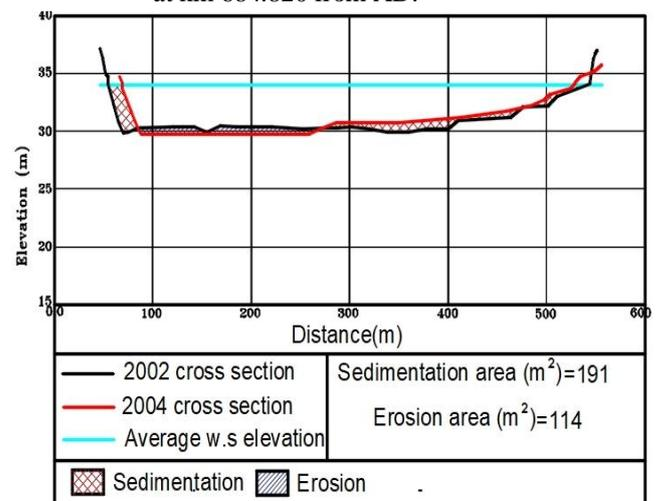
**Fig 9.** The deposition and scour at a cross-section at km 685.305 from AD.
