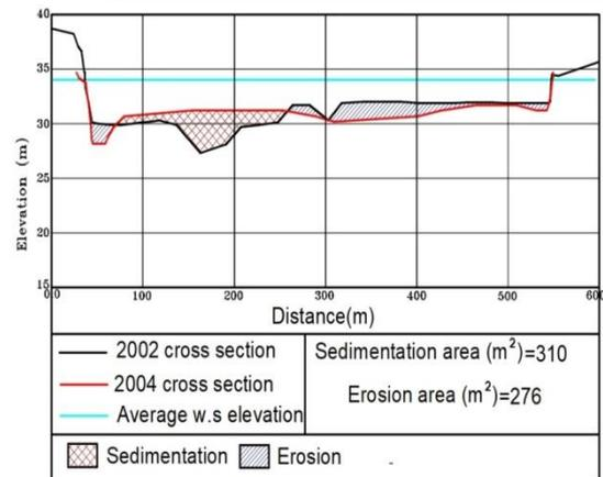
**Fig 7.** The deposition and scour at a cross-section at km 684.450 from AD.
