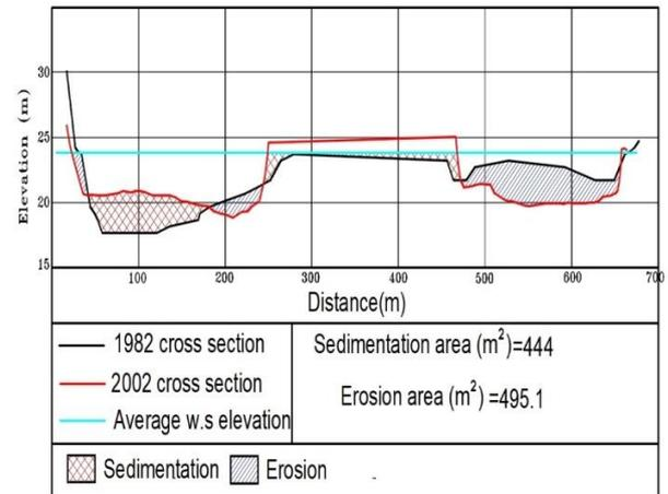
**Fig 11.** The deposition and scour at a cross-section at km 808.870 from AD.
