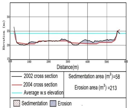
**Fig 14.** The deposition and scour at a cross-section at km 809 from AD.
