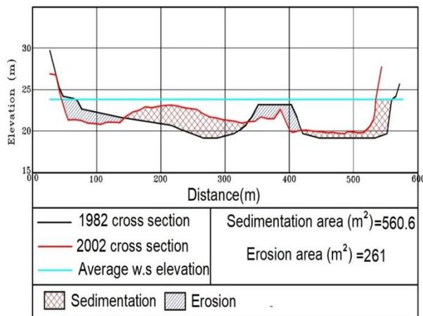
**Fig 13.** The deposition and scour at a cross-section at km 808.27 from AD.
