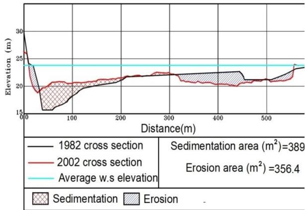
**Fig 10.** The deposition and scour at a cross-section at km 808.350 from AD.
