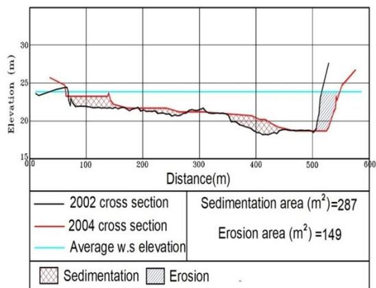
**Fig 15.** The deposition and scour at a cross-section at km 810.705 from AD.
