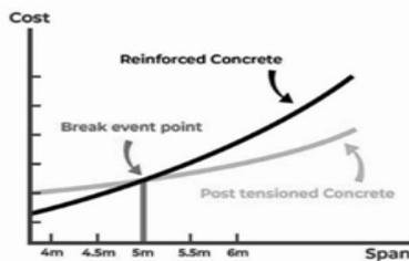
**Fig 6:** Exponential saving for span < 5 m
