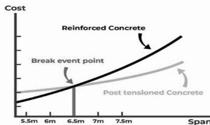
**Figure 7:** Exponential saving for span  $6.5 > m$
