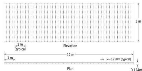
**Fig 1:** Dimensions of GFRG Panel
