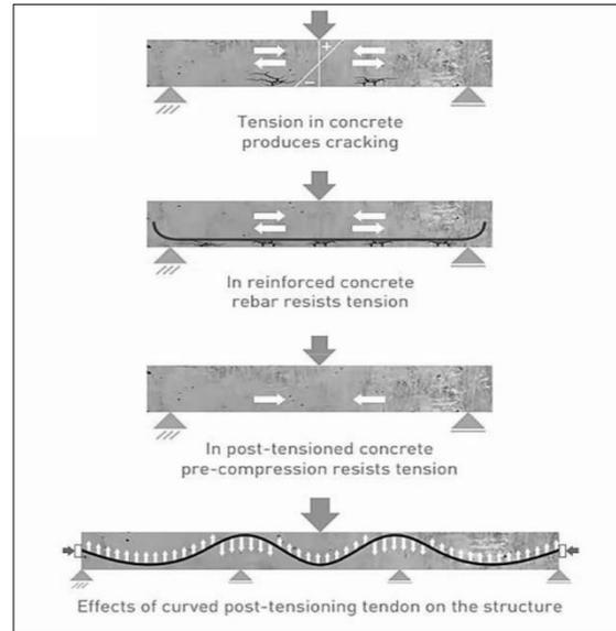
**Fig 2:** Effect of post tensioning on the structure
