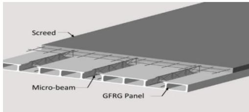
**Fig 3:** GFRG floor slab with micro beam and screed
