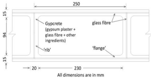
**Fig 2:** Enlarged View of a Typical Cell
