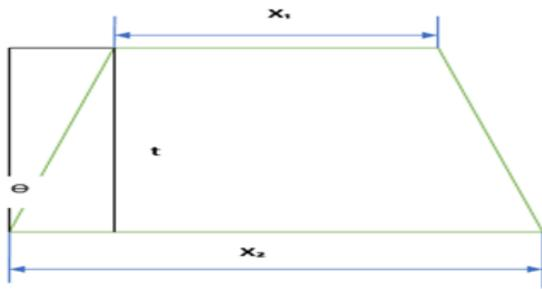
Fig.5: Schematic diagram for taper angle measurement
