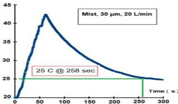
A smaller droplet size has been used while keeping all previous conditions of fig. no. (6) constant, the extinguishing time has been enhanced to be 258 sec
