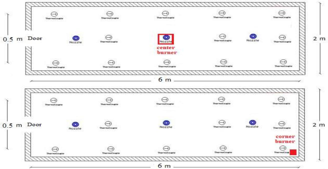
Figure 1. "Plan of hanger model"
