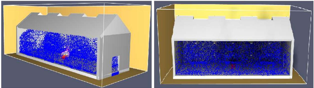
Figure 10. “Activation of water mist on fire at center “
