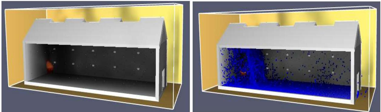
Figure 11. “Activation of water mist on fire at corner “
