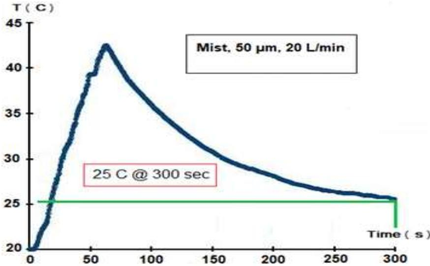
In this fig. no. (6), once applying the water mist fire suppressing system to the same model of previous fig. no. (5), a pronounced effect has been occurred, and finally the fire is extinguished @ 300 sec.
