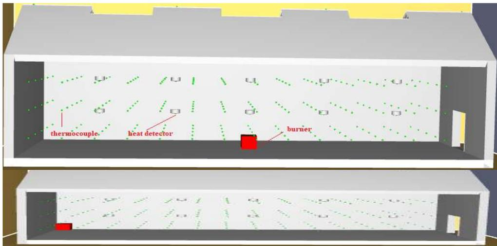
Figure 3. "Schematic 3D view of hanger model (FDS)"
