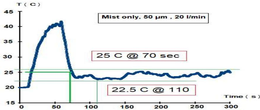
Figure 9. “Average Temperature of using water mist only (Q= 500 kW/m<sup>2</sup>, q mist= 20 l/min, Di= 50 μm)”
