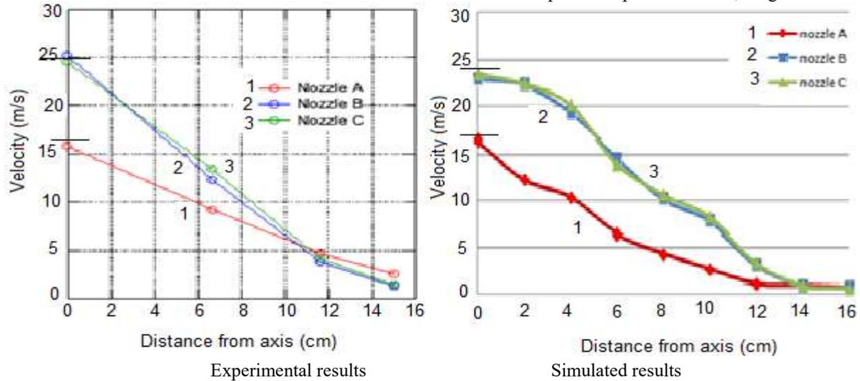
Figure 4. “Experimental [13] and simulated data for nozzles A, B, and C”
