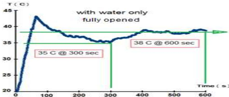
This figure reflects the poor effect of using water only on the fire extinguishing, during 600 sec the sprayed water couldn't extinguish the fire
