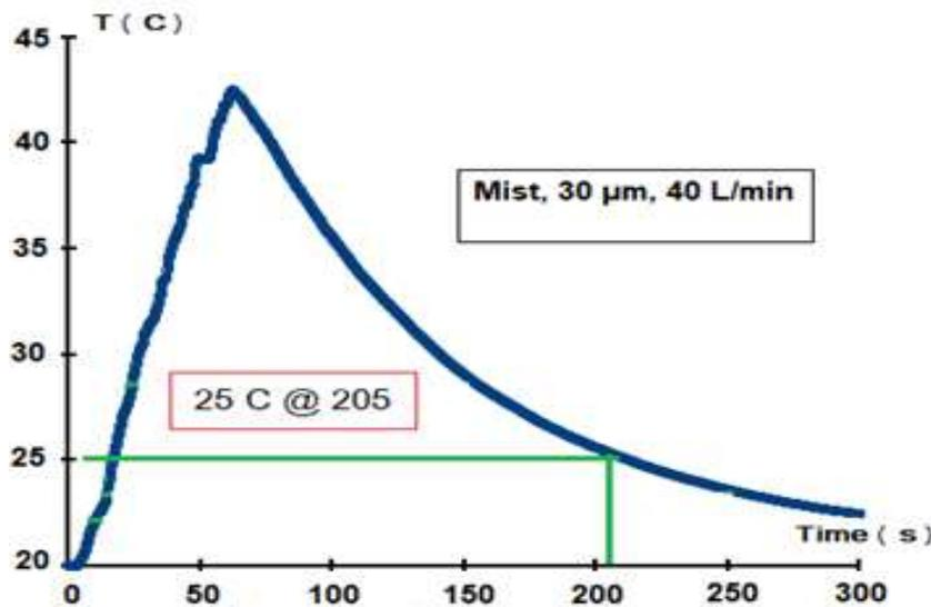
After double the quantity of flow rate amount to be (40 l/m), maintaining all conditions the same as previous fig. no. (7), an enhancement in time of fire extinguishing has been occurred by more than 50 sec to be reached 205 sec
