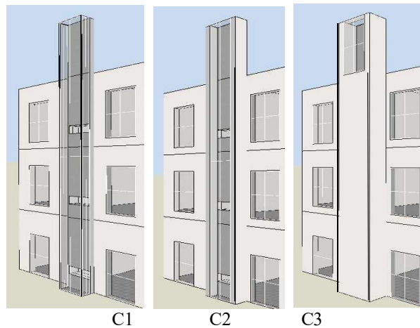
FIGURE 23. 3D model for solar chimney on each case
