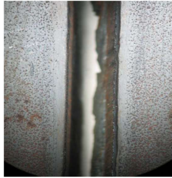
Figure 7: Showing widest kerf width at the lowest cutting speed (300mm/min)
