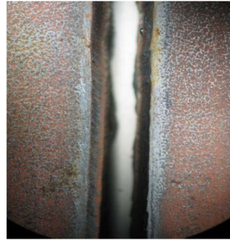
Figure 8: Showing narrowest kerf width at highest cutting speed(700mm/min)
